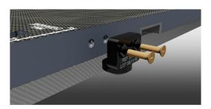
Mount the Loxon blocks to the side of the base plate using the plastic countersunk M5 x 20 screws and a screwdriver.
