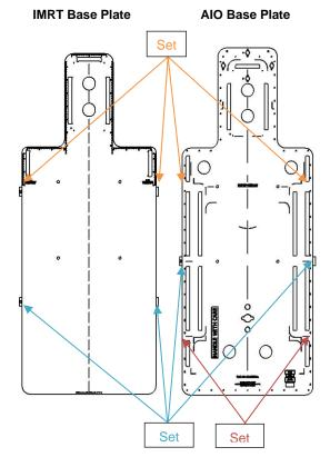
When only one set of Loxons is used, combine it with a Table Fix or a 2-pin indexing bar and an adapter plate. Information on these other parts can be found in the respective 'instructions for use' and the Orfit website:
