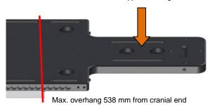
Below sag and creep results at conditions of maximum overhang, force at cranial end and 21°C.
