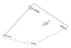
The clamps can cover treatment table widths from maximum 566 mm (22,28 inches) to a minimum of 406 mm (15,98 inches) depending on the position the cylinder is in. In position A the range is between 566 and 468 mm while in position B the table width can be between 506 and 408 mm.
