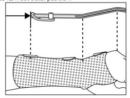
**11.** For a few seconds, heat the underneath of the ORFITUBE ADJUSTER as well as the attachment location on the orthosis with a heat gun (be careful for overheating).
